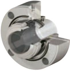
This medium- to high-pressure seal features a high balance face that meets the lowest light hydrocarbon emissions level: less than 500 ppm. Designed to suppress flashing and minimize heat generation.
